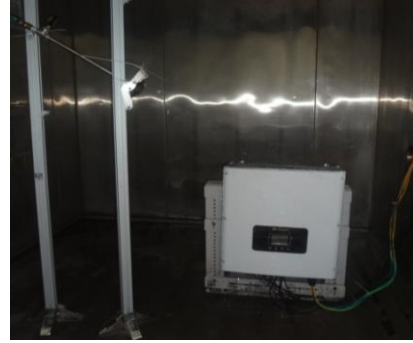
Photo 8 Water spray test photo
