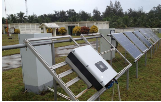
Photo 13 350M exposure field of inverter
